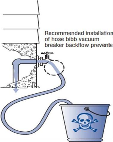
Recommended installation of hose bibb vacuum breaker backflow preventer
